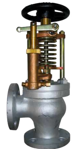
QUICK CLOSING ANGLE VALVES, F7399-A JIS 10K CAST STEEL BODY, STAINLESS STEEL TRIM -WITH DNV-GL CLASS CERTIFICATE
